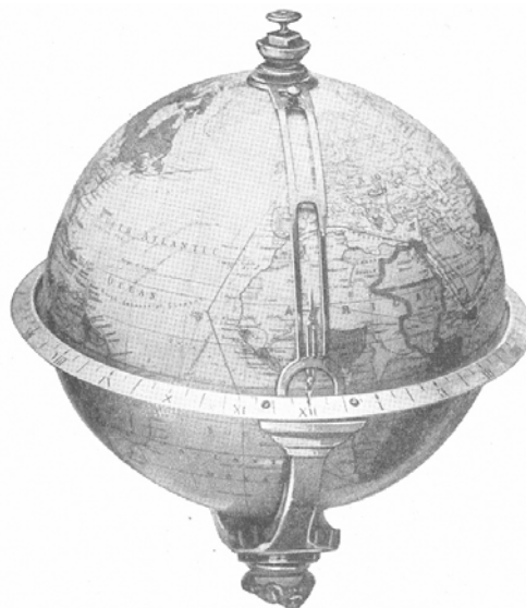
The globe is turned by clock-work and tells what time it is at any given moment in any part of the world.
